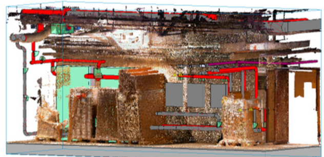
Location of the new domestic hot water production system in the point cloud
