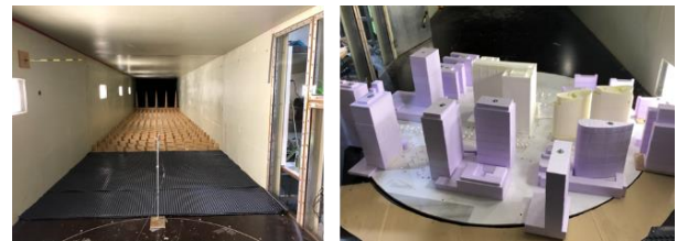
Figure 6a Modification of wind forces – 6b. wind tunnel tests
