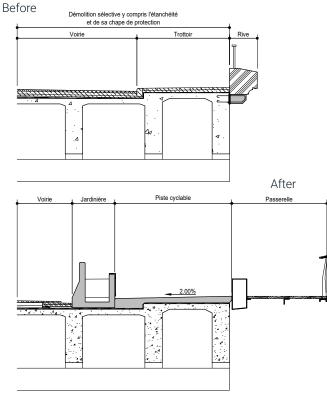
The metal box is simply supported along its length on the edge beam of the existing structure, while a recess is made at the piers and abutment. The steel box-girder is simply supported along its length on the edge beam of the existing structure, and embedded at the piers and abutments. The aim of this arrangement is to avoid overloading the existing structure's edge beam, which does not have sufficient reserves.
