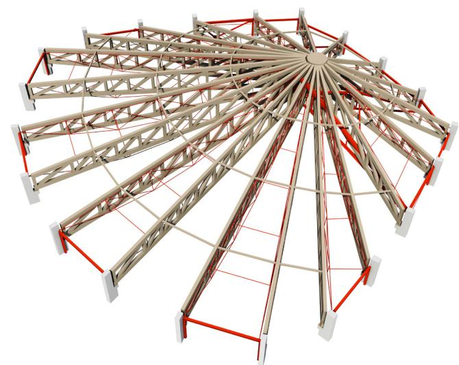
All the elements constituting the frame must be able to be transported by hand or via spreaders suspended from the primary frame (limitation to 1 ton).
