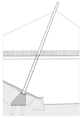
Cable-stayed steel bridge 90 m long, with a 50 m central span between two inclined pylons.
